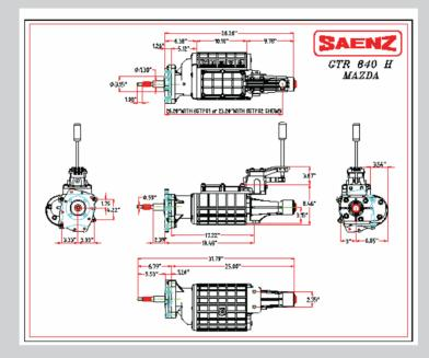
This drawing shows a GTR840 adapted for RX7 Mazda engine, any other adaptor, input shaft length could be made upon request.
